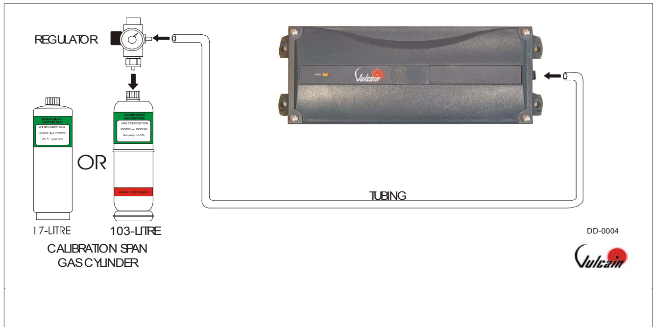
Figure II – 301IRFS Calibration equipment setup
